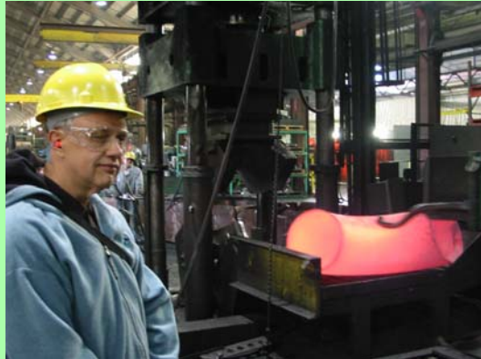
NACE Portland Section Vice Chairman Bernie Covino watching a 16 inch elbow being forged.
